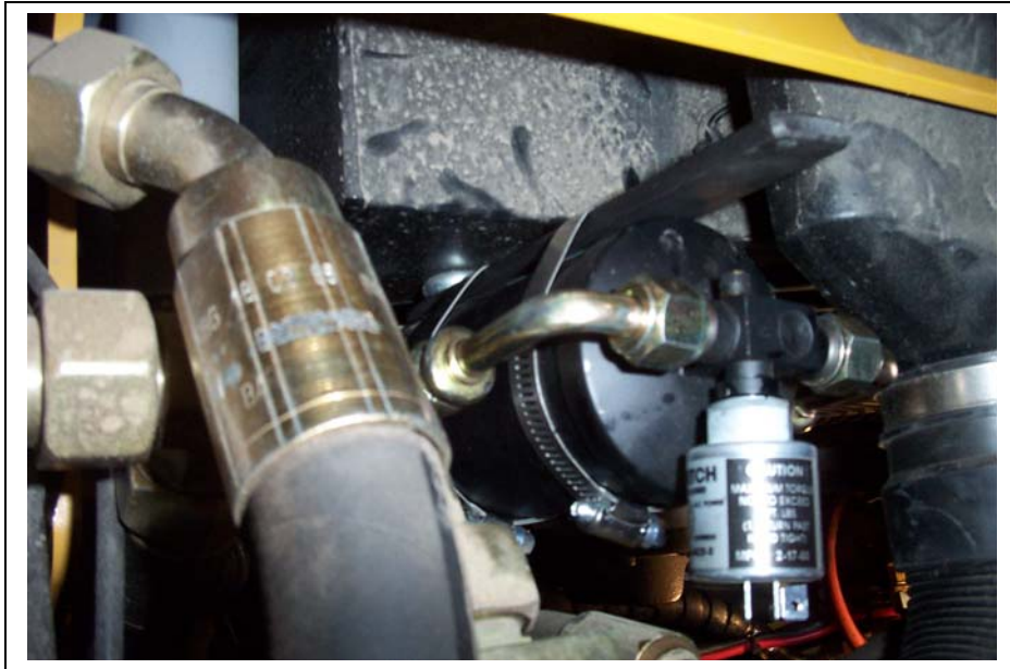
Receiver drier with trinary switch mounted on fan shroud
