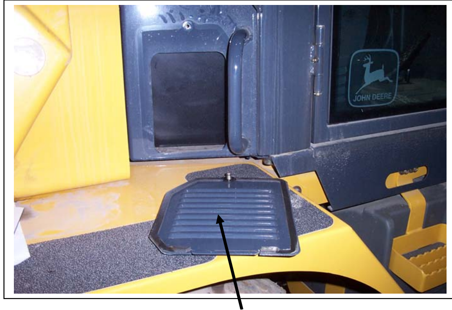
Outside air intake louvered door off.
