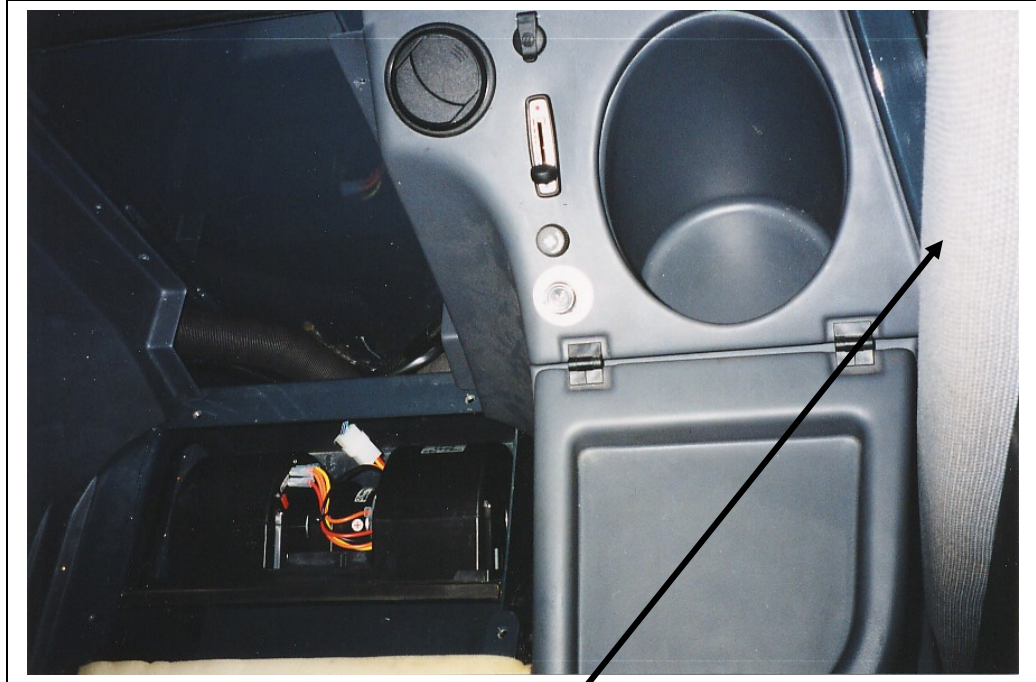
This cover is hollow and could accommodate a flex hose and louver mounted at head level.
