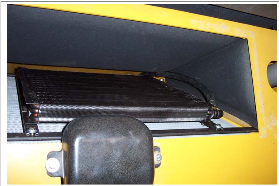
Condenser in place on intake side of radiator
