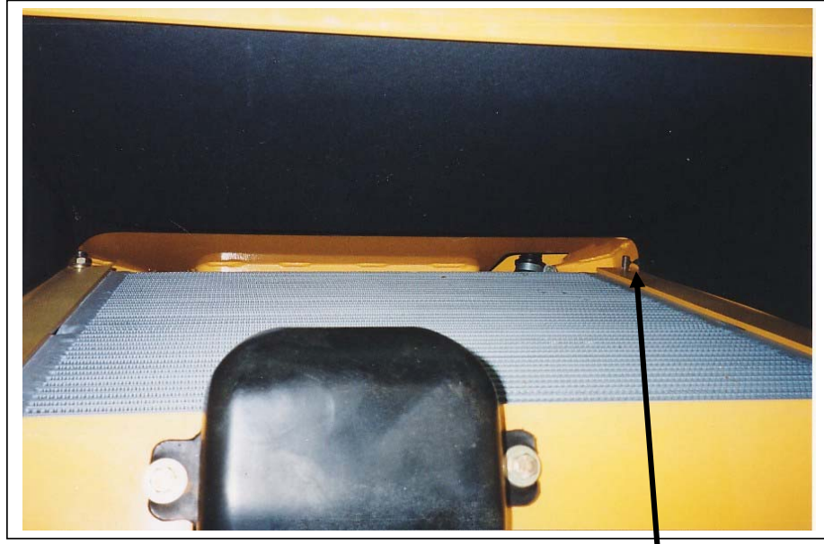
View of condenser mounting area on the intake side of the radiator
