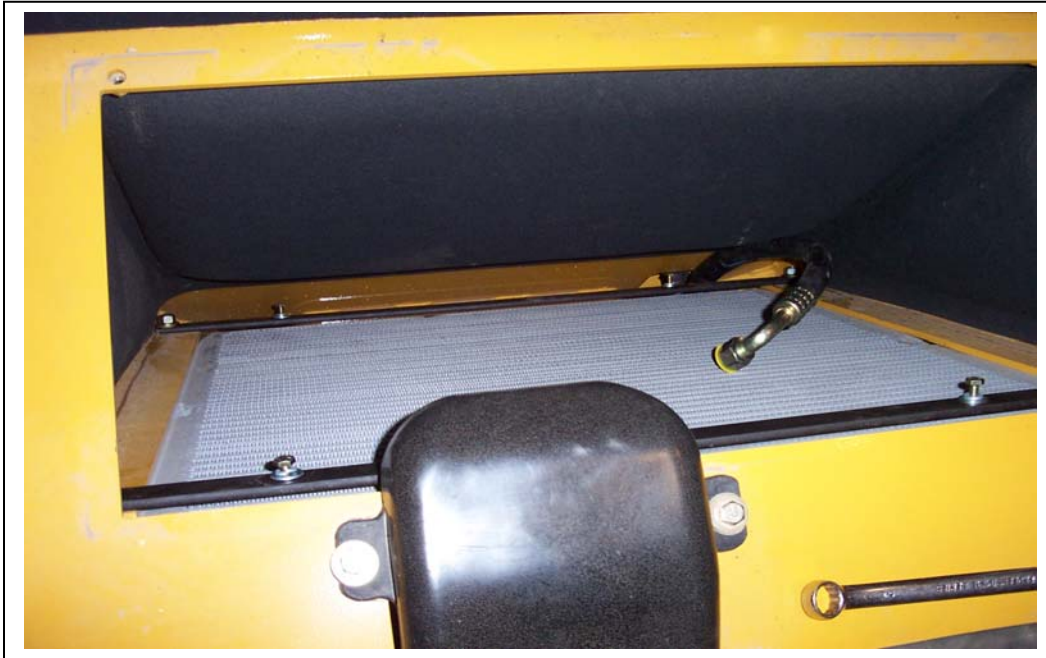
Condenser mount brackets installed across the radiator face.
