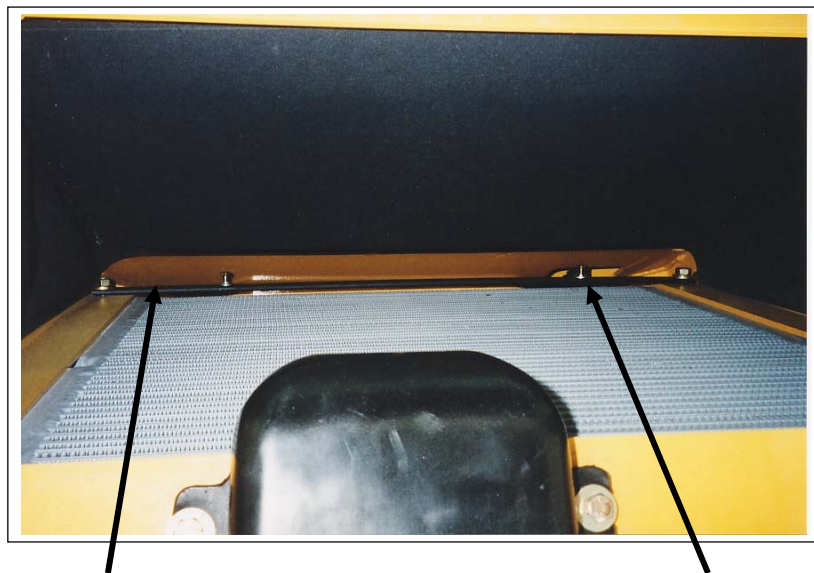
Lower condenser mount bracket installed
